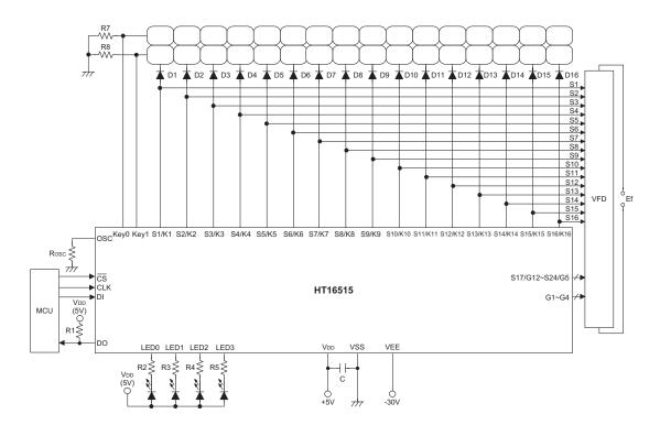
Note:  $R_{OSC}$ =82 $k\Omega$  for oscillator resistor
