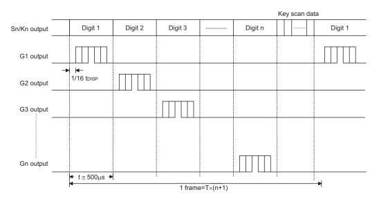
Note: One cycle of key scanning consists of two frames, and data of  $16\times2$  matrixes is stored in the RAM.
