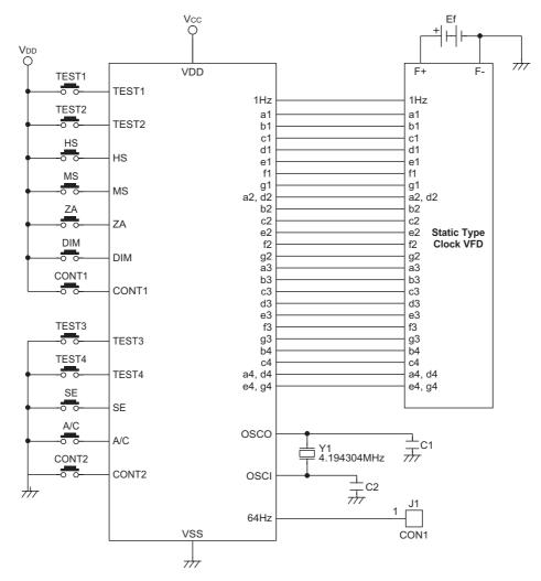
Note: Capacitors C1 and C2 can adjust the frequency accuracy
