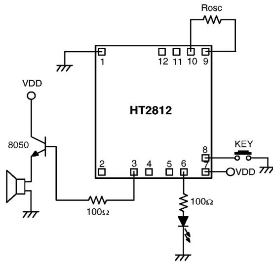
\* The IC substrate should be connected to VDD in the PCB layout artwork.
