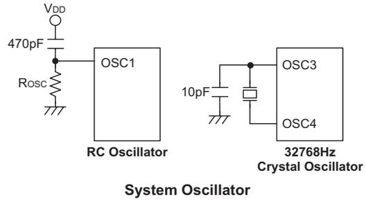
recommended to turn on the quick oscillating function at power on until the RTC oscillator is stable, and then turn it off after 2 seconds to reduce power consumption.
