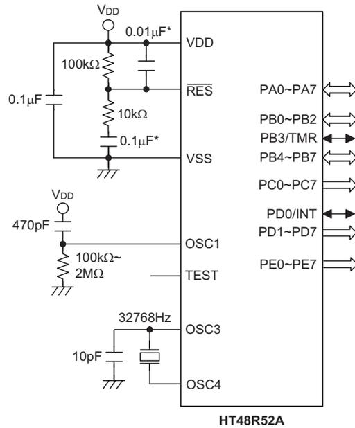
Note: The resistance and capacitance for the reset circuit should be chosen in such a way as to ensure that VDD is stable and remains within a valid operating voltage range before bringing RES high.
