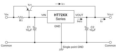
$$R_1 = \frac{V_{BE1}}{I_{REG} - \frac{I_{C1}}{(1+\beta)}}$$
