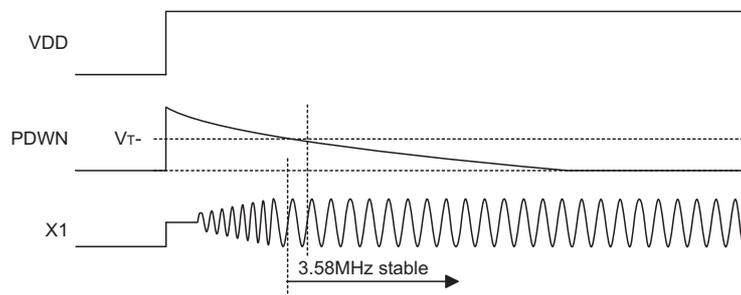
Note: reference  $C_1=0.1\mu\text{F}$   $R_1=81\text{k}\Omega$
