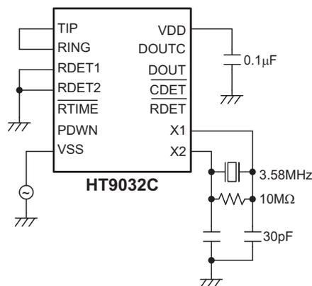
Supply current testing: All, except PDWN and  $\overline{RTIME}$ , unwired pins are left floating.
