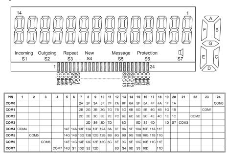
**Note** The recommended optimal operating voltage for the LCD panel is 0.93VDD and choose 3V/4.5V LCD panel to fit 2-pcs or 3-pcs battery where VDD is 3.2V/4.8V.
