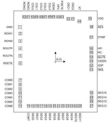
\* The IC substrate should be connected to VSS in the PCB layout artwork.
