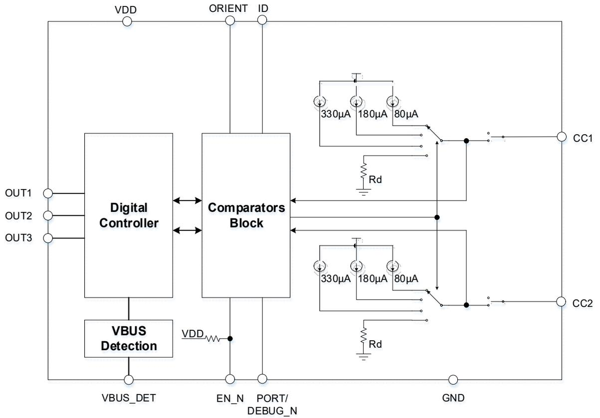
Figure 3. HUSB320-AA000 Functional Block Diagram
