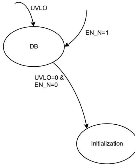
Figure 4. Dead Battery Timing
