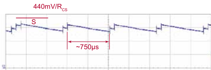
Fig.2. Short-circuit inductor current.
