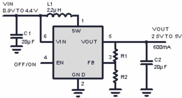
\*LOCATE COMPONENTS CLOSE TO THE PIN
