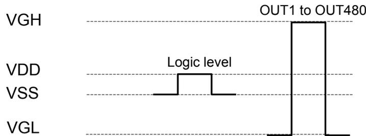
The logic levels of CPV, L/R, OE, /XAO, MODE1, MODE2, MODE3, EVEN, SGOFF, STV1 and STV2 have to swing between VDD for “H” and VSS for “L”.
