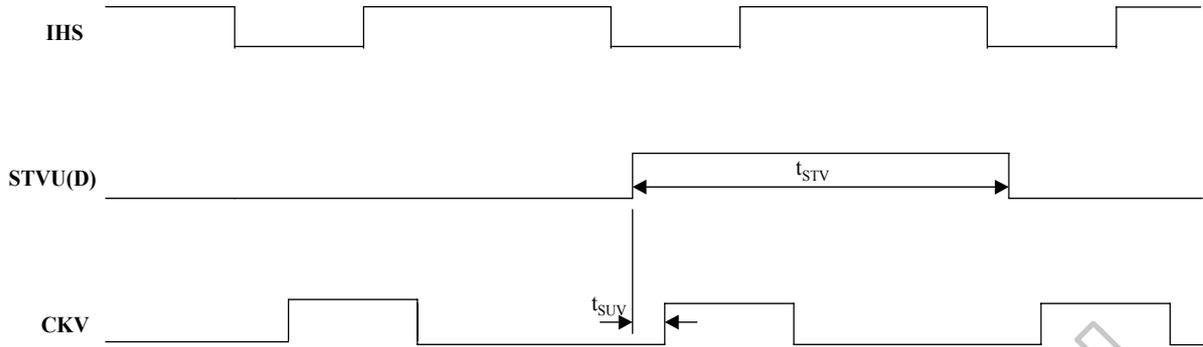
9.6 IHS and vertical control timing waveform (for the case of UDC="H")
