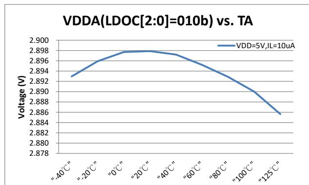
Figure 6.7-5 VDDA(010b) vs. Temperature
