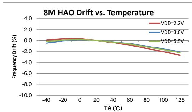
Figure 6.3-4 HAO(8.0MHz) vs. Temperature
