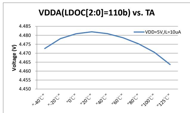
Figure 6.7-6 VDDA(110b) vs. Temperature
