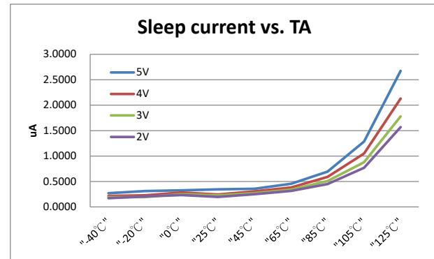
Figure 6.4-2  $I_{LP3}$  vs. Temperature
