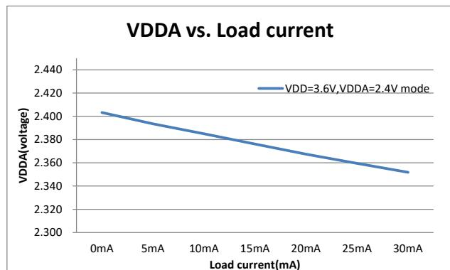
Figure 6.7-7 VDDA vs. Load current
