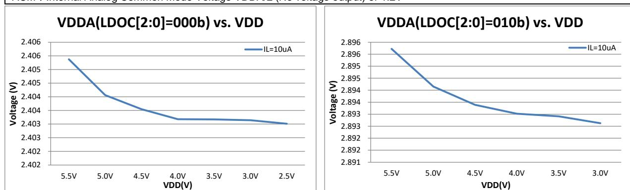
Figure 6.7-1 VDDA(000b) vs. VDD
