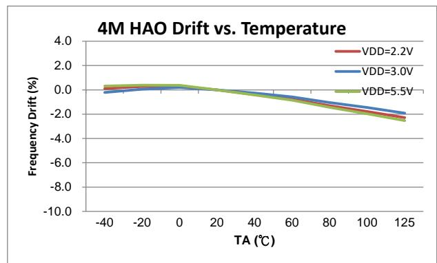
Figure 6.3-3 HAO(4.0MHz) vs. Temperature
