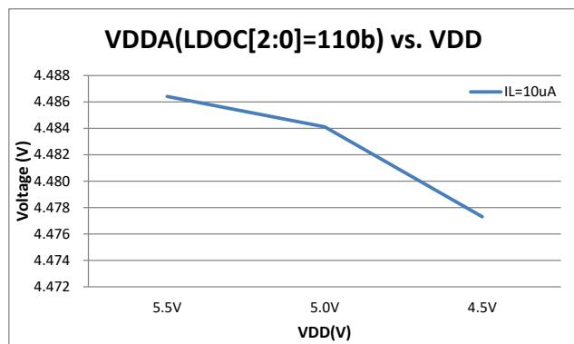
Figure 6.7-3 VDDA(110b) vs. VDD
