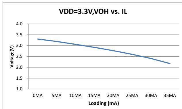
Figure 6.5-1  $V_{OH}$  vs.  $I_{OH}$
