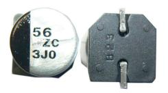
Type HZC hybrid capacitors are a combination of solid polymer aluminum technology with wet aluminum electrolytic technology. This results in a surface mount capacitor with a 4,000 hour life, low leakage current, high voltage capability, very low esr and small case sizes. They are ideal for high temperature and high reliability PC board designs. The vertical cylindrical cases facilitate automatic mounting and feature high reflow soldering temperature capability. Type HZC is RoHS compliant.
