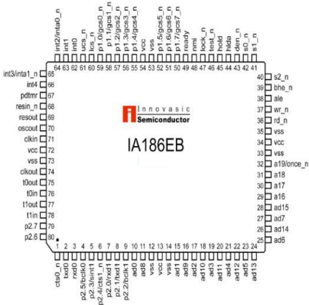
Figure 4. IA186EB 80-Pin PQFP Package Diagram
