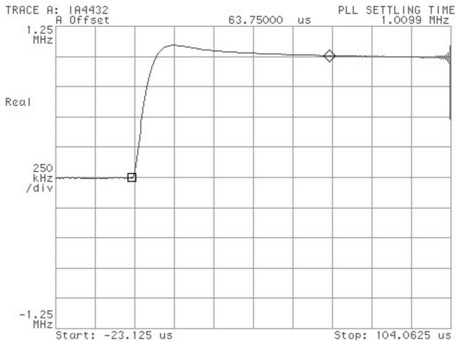
Figure 42: Synthesizer Settling Time for 1MHz Jump settled within 10kHz
