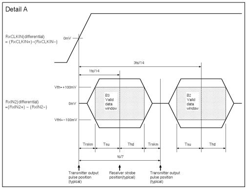
**Note:** Tsu and Thd are internal data sampling window of receiver. Trskm is the system skew margin; i.e., the sum of cable skew, source clock jitter, and other inter-symbol interference, shall be less than Trskm.
