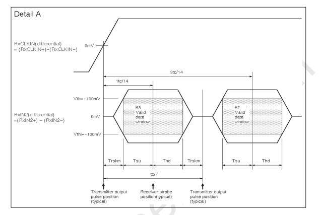
**Note:** Tsu and Thd are internal data sampling window of receiver. Trskm is the system skew margin; i.e., the sum of cable skew, source clock jitter, and other inter-symbol interference, shall be less than Trskm.
