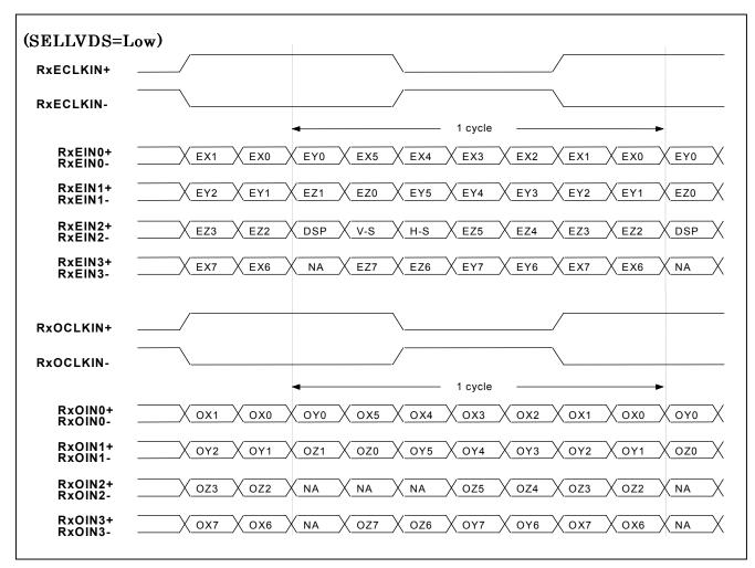
Note: X/Y/Z data 7: MSB, X/Y/Z data 0: LSB, DSP = DSPTMG, V-S = Vsync, H-S = Hsync
