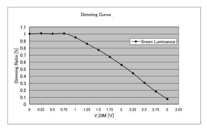
**Note :** This curve depends on the temperature and total running time of the backlight.
