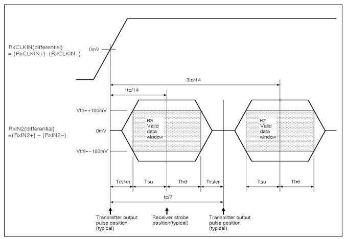
**Note:** Tsu and Thd are internal data sampling window of receiver. Trskm is the system skew margin; i.e., the sum of cable skew, source clock jitter, and other inter-symbol interference, shall be less than Trskm.
