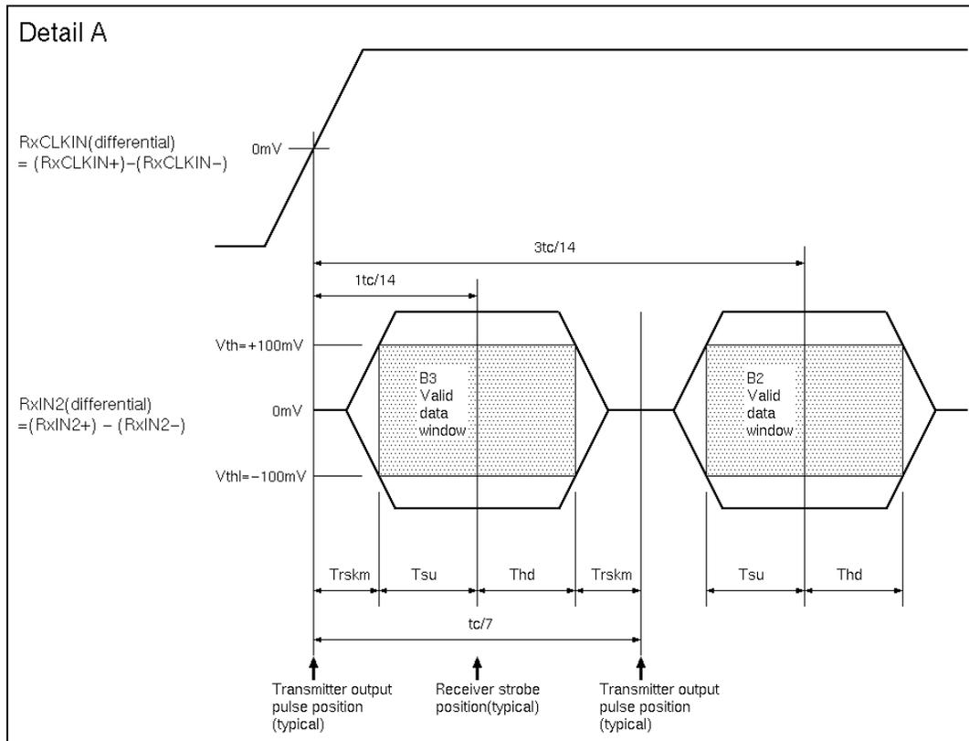
**Note:**  $T_{su}$  and  $T_{hd}$  are internal data sampling window of receiver.  $T_{skm}$  is the system skew margin; i.e., the sum of cable skew, source clock jitter, and other inter-symbol interference, shall be less than  $T_{skm}$ .
