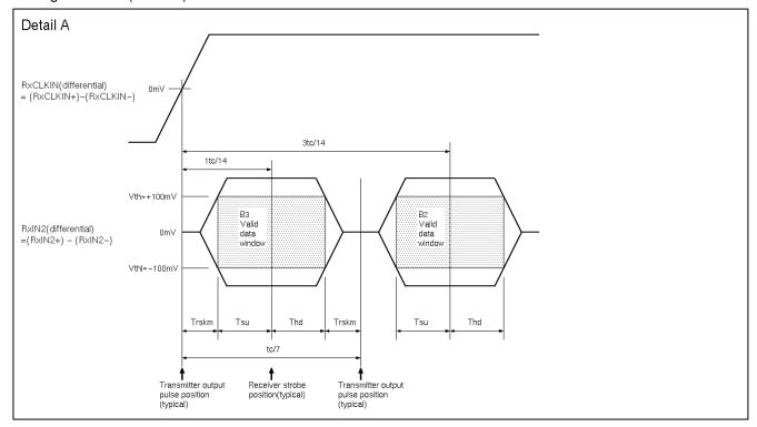
**Note:** Tsu and Thd are internal data sampling window of receiver. Trskm is the system skew margin; i.e., the sum of cable skew, source clock jitter, and other inter-symbol interference, shall be less than Trskm.
