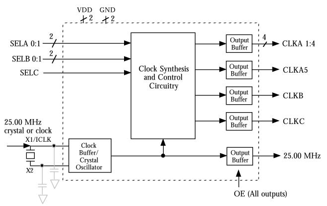
Optional crystal capacitors are shown and may be required for tuning of initial accuracy (determined once per board).
