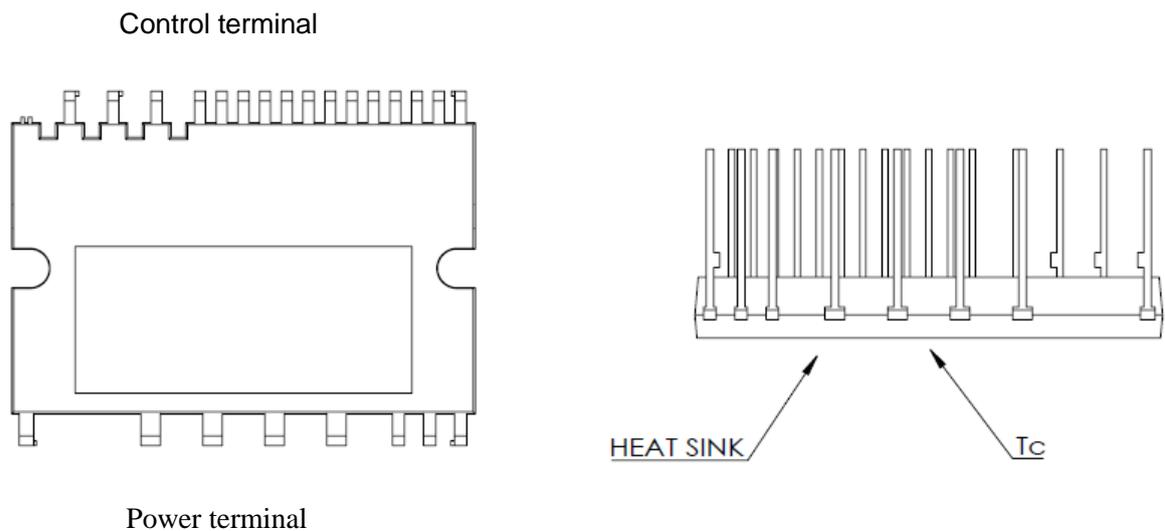
Figure 4.  $T_c$  Measurement Point
