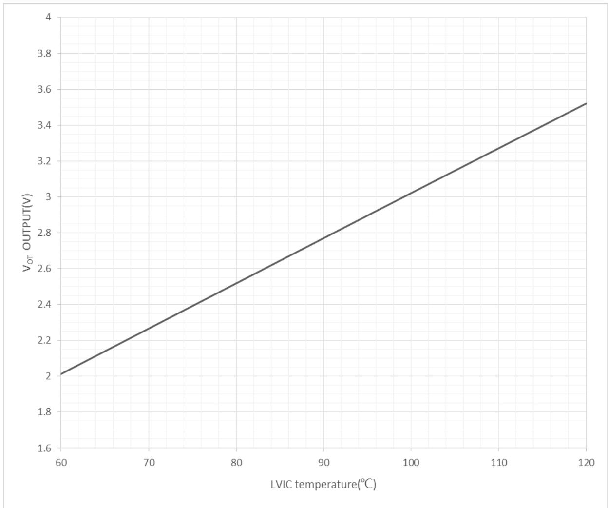
Figure 7. V<sub>OT</sub> output characteristics
