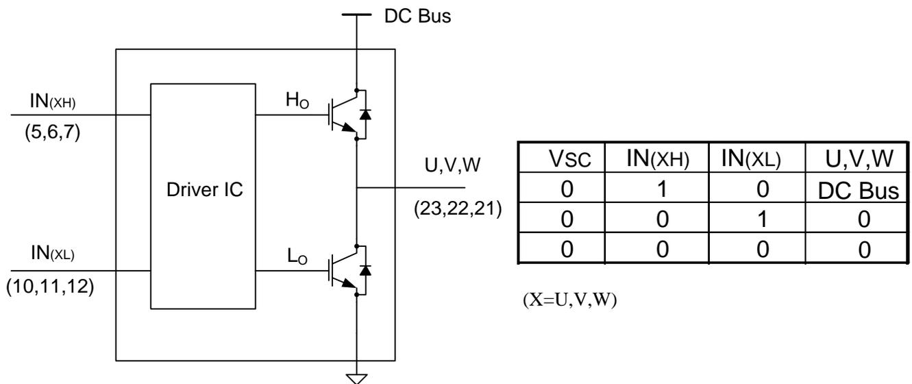
Figure 10. Input/Output Signal Circuit
