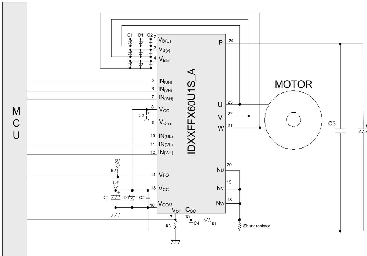
Figure 13. Typical Application Circuit Interface Example without Photo-Coupler
