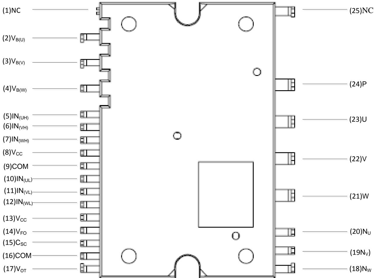
Figure 2. Pin Configuration
