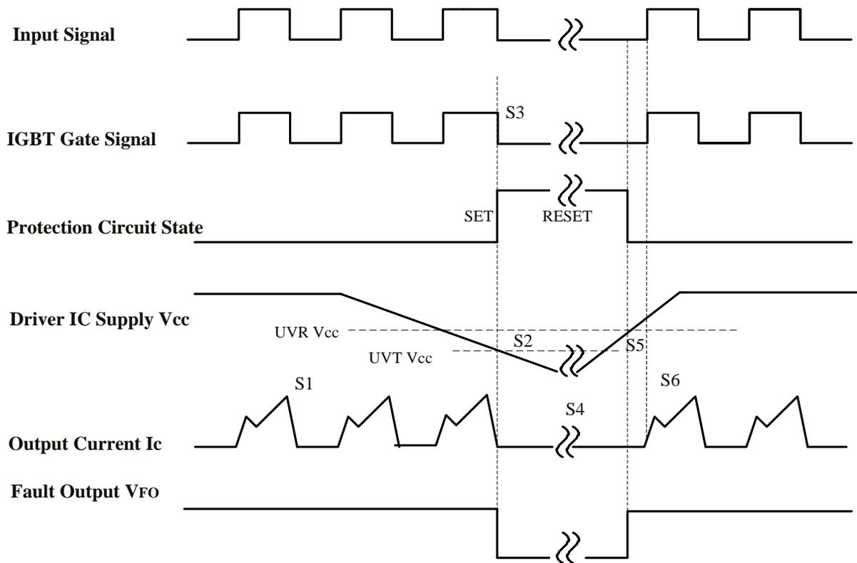
Figure 12. Timing Chart of Under-Voltage Operation
