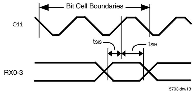
Figure 7. Serial Outputs and External Control
