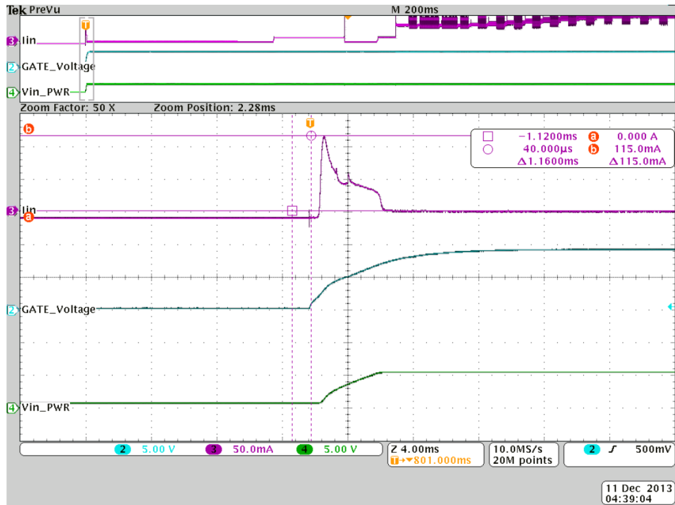
Figure 4. Inrush Current Limit Operation
