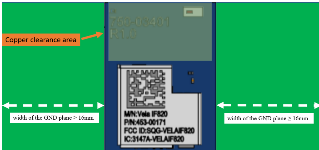
Figure 15: Integrated antenna variant layout suggestion example
