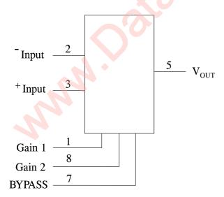
$\begin{aligned} &Pin \ 4 = GND \\ &Pin \ 6 = Supply \ Voltage \ V^{+} \end{aligned}$
