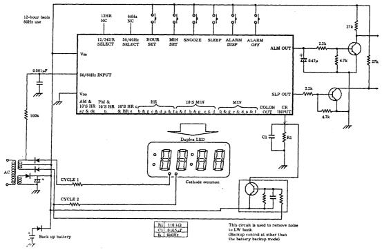
SAMPLE APPLICATION CIRCUIT FOR CLOCK USE (-power supply)
