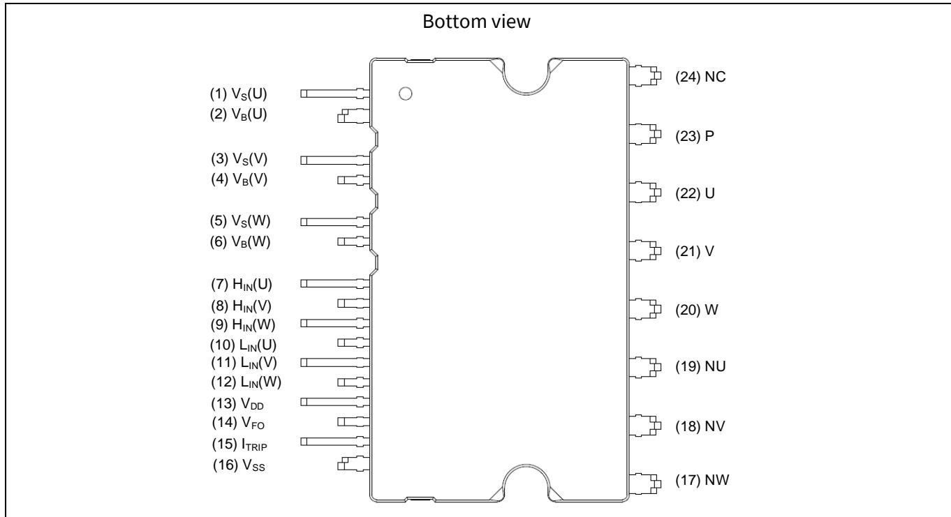
**Figure 2 Pin configuration**
