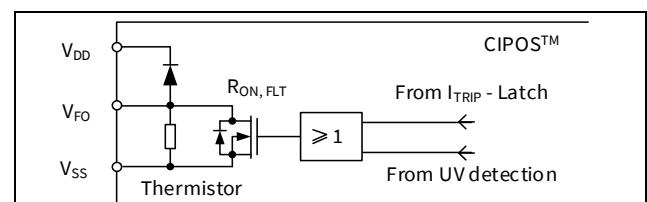
**Figure 5** Internal circuit at pin V<sub>FO</sub>
