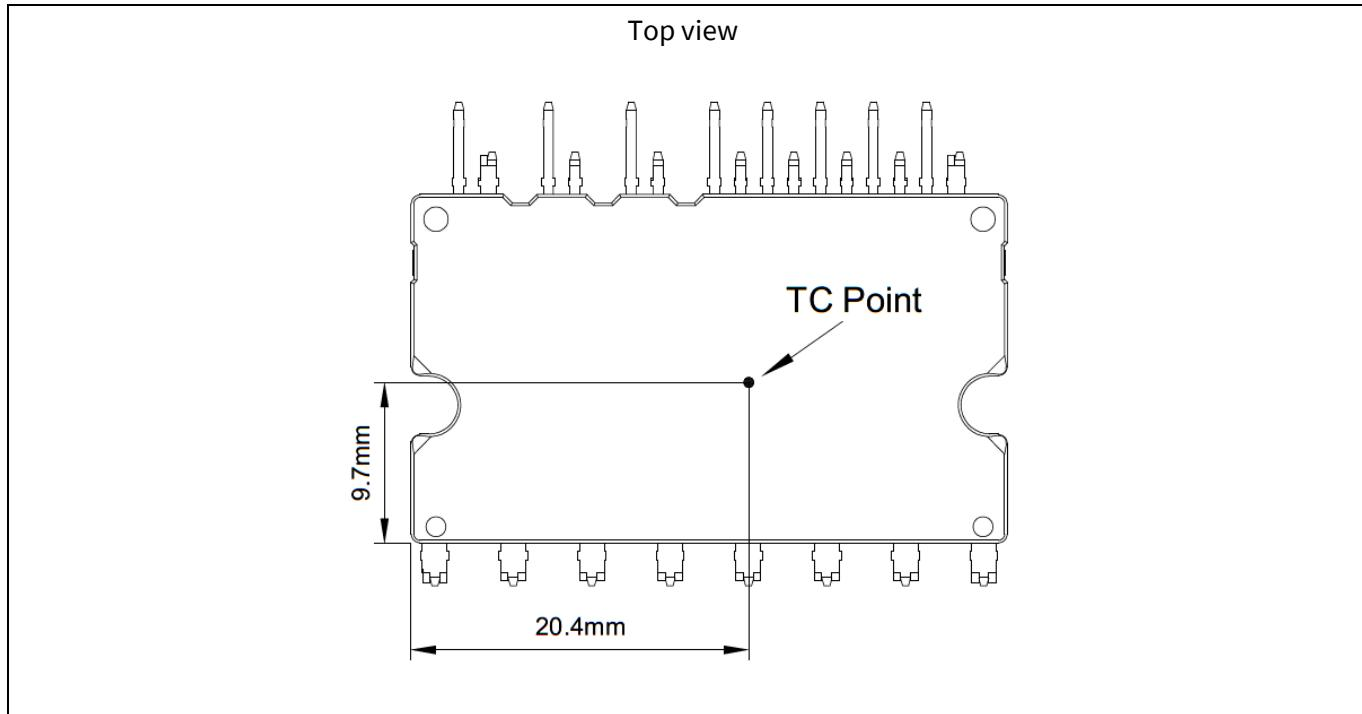
Figure 7  $T_c$  measurement point<sup>1</sup>
