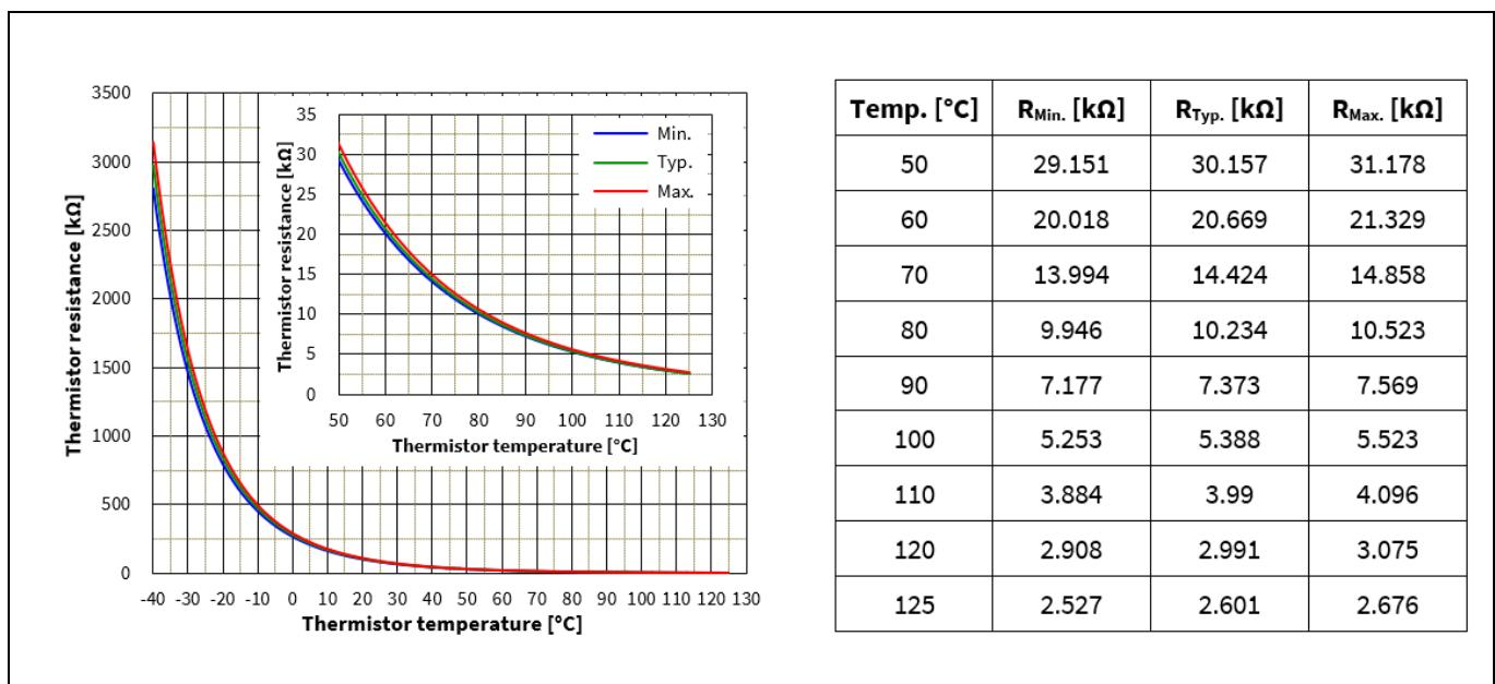
**Figure 6 Thermistor resistance – temperature curve and table**
