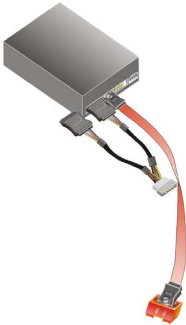
Figure 4-13: SATA Power Drive Connection
