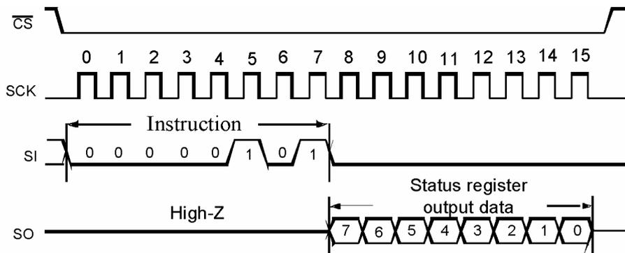
The RDSR (read status register) instruction provides access to the status register. The status register may be read at any time, even during a write cycle.
