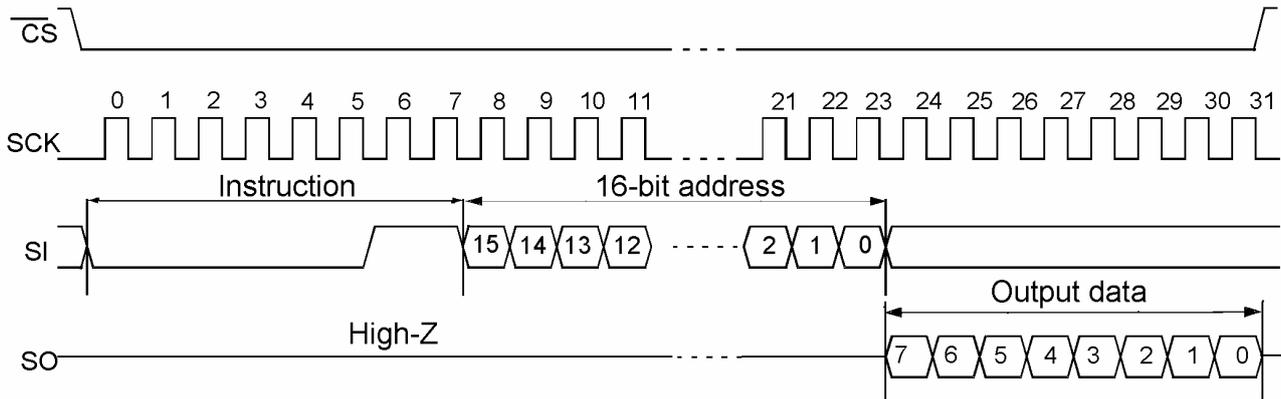
There are six 8-bit instructions available for executing of read/write operation. The feature of IN25AA080N, IN25AA080D (IN25AA160N, IN25AA160D) is that 6 (5) higher address bits are insignificant (have to be ignored).
