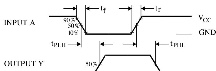
**Figure 1. Switching Waveforms**
