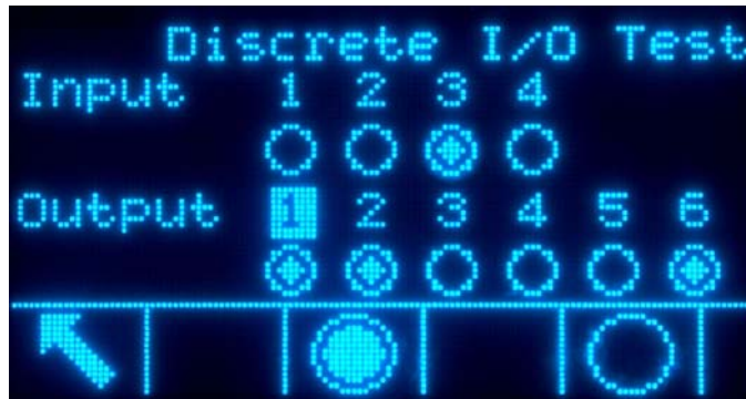
Figure 4-7: Discrete I/O Test Screen
