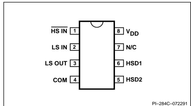
Figure 2. Pin Configuration.
