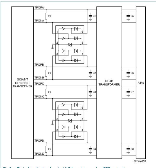
Fig 5. Typical application for gigabit Ethernet transceiver ESD protection
