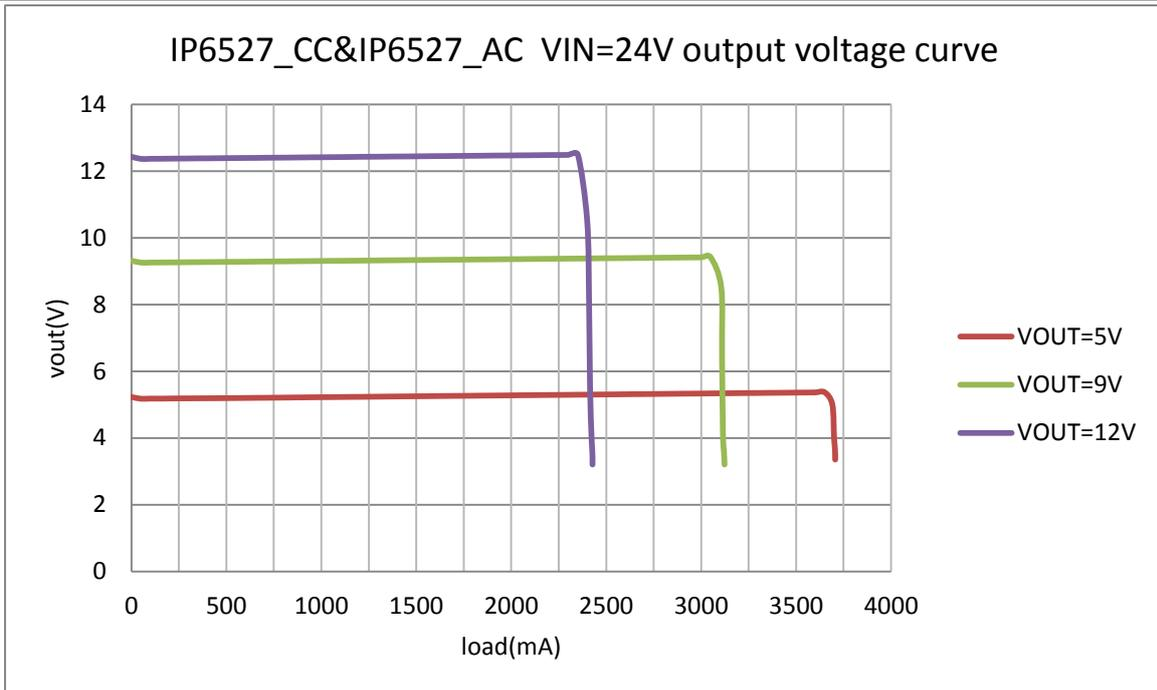
Figure 4. IP6527\_C Vout-lout curve when VIN=24V
