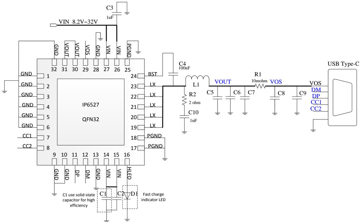
Figure 6. IP6527\_C Type-C output ports fast charge application schematic diagram
