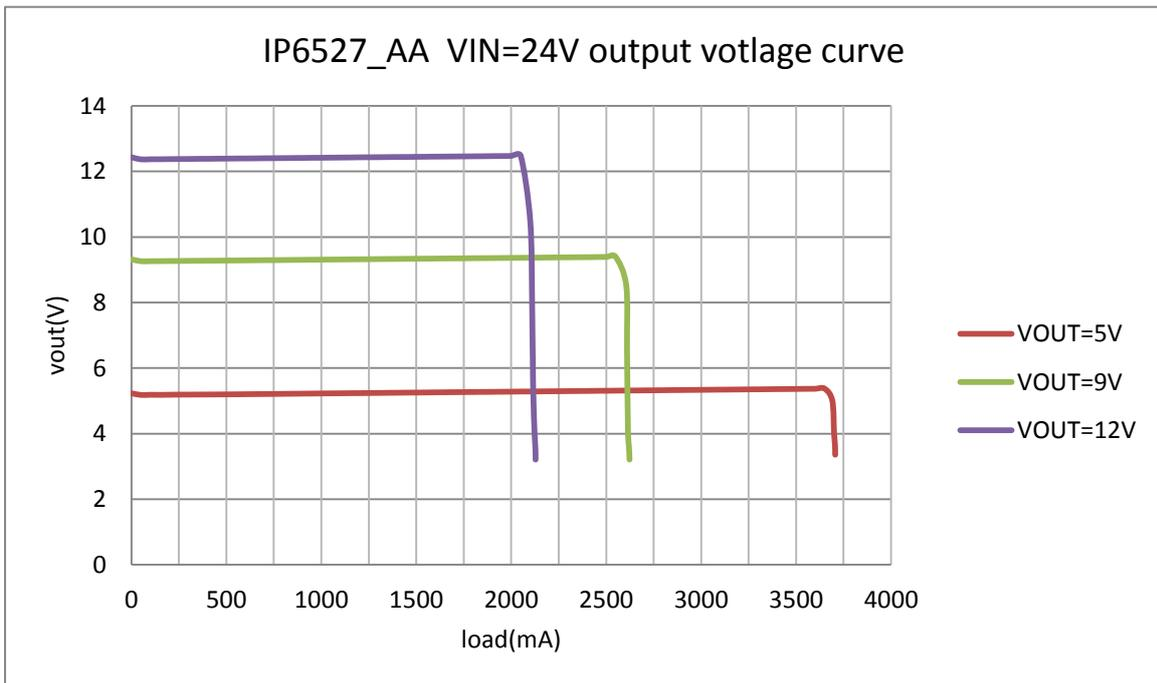
Figure 5. IP6527\_A Vout-lout curve when VIN=24V
