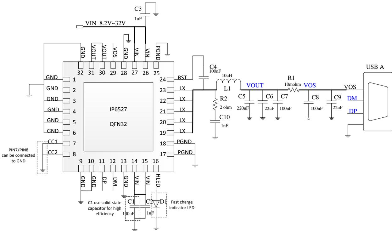
Figure 7. IP6527\_A USB A output ports fast charge application schematic diagram
