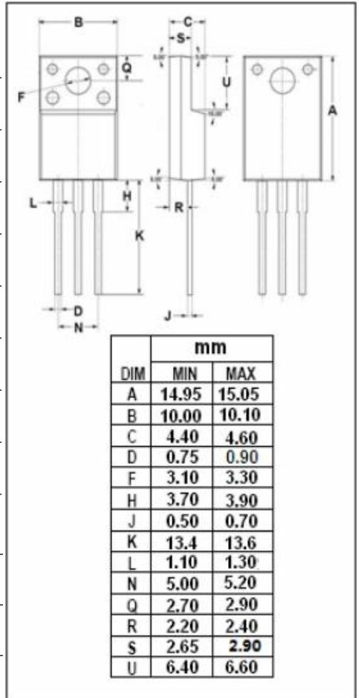
**isc N-Channel MOSFET Transistor**
