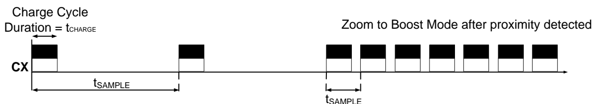
Figure 6.5 LP Modes: Charge cycles
