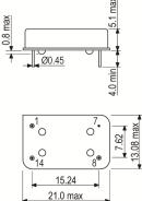
Pin Connections 1. Standby Operation 7. GND 8. Output 14. +Vs
