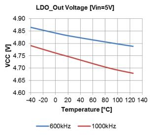
Figure 18: LDO\_Out Voltage in dropout mode
