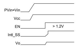
Figure 5: Recommended startup for Normal operation
