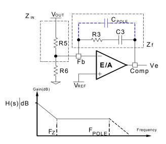
Figure 26: Type II compensation network and its asymptotic gain plot
