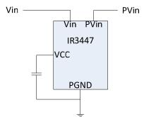
Figure 15: Internally Biased Configuration
