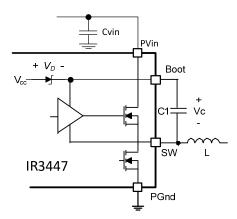
Figure 24: Bootstrap circuit to generate Vc voltage
