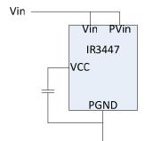
Figure 16: Internally Biased Single Supply Configuration
