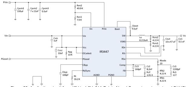
Figure 29: Application circuit for a 12V to 1.2V, 21A Point of Load Converter using external 5V VCC
