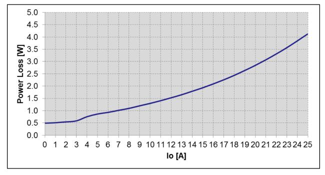
Figure 41: Power Loss versus load current
