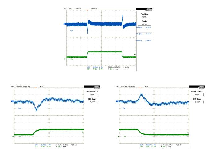
Figure 37: Vout Transient Response, 2.5A to 10.0A step at 2.5A/uSec CH2:Vout, CH4:Iout (10A/V)
