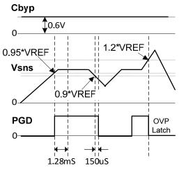
Figure 19: PGood Timing Diagram
