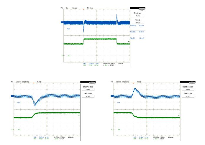
Figure 38: Vout Transient Response, 17.5A to 25A step at 2.5A/uSec CH2:Vout, CH4:lout (10A/V)
