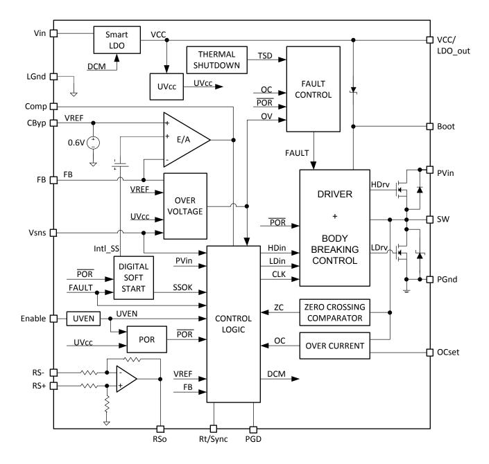
Figure 3: IR3447 Simplified Block Diagram
