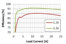
Figure 2: Efficiency [Vin=12V, Fsw=600kHz]
