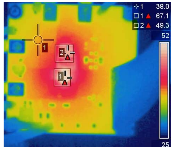
Figure 22: Thermal Image at VIN = 19V, IOUT = 6A (IR3473: 67°C, Inductor: 49°C, PCB: 38°C)
