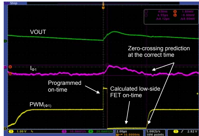
Figure 41: PS2 Active Diode Emulation Mode
