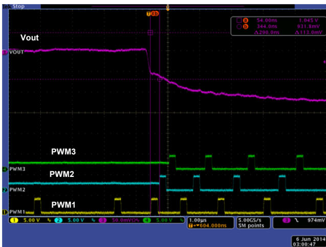
Figure 39: Phase Add 1\Phi \rightarrow 3\Phi
