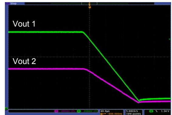
Figure 20: MPoL Tracking Shutdown
