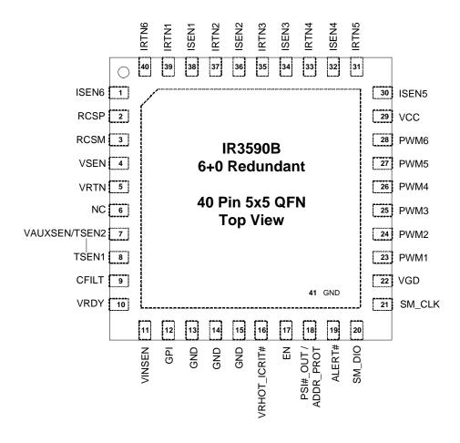
Figure 1: IR3590B Package Top View
