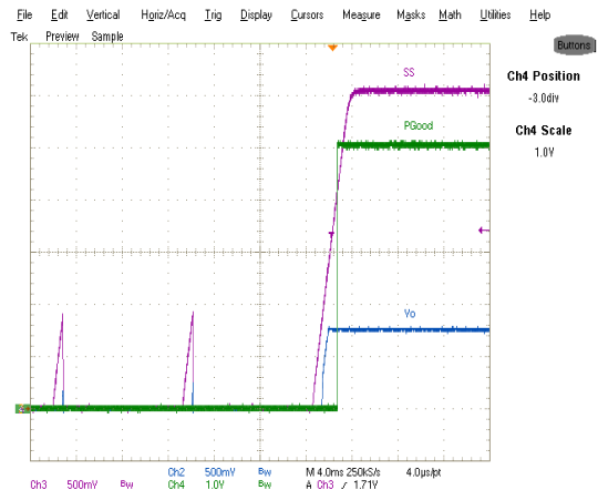
Fig. 21: Short (Hiccup) Recovery Ch 2 :V out , Ch 3 :V SS , Ch 4 :PGood
