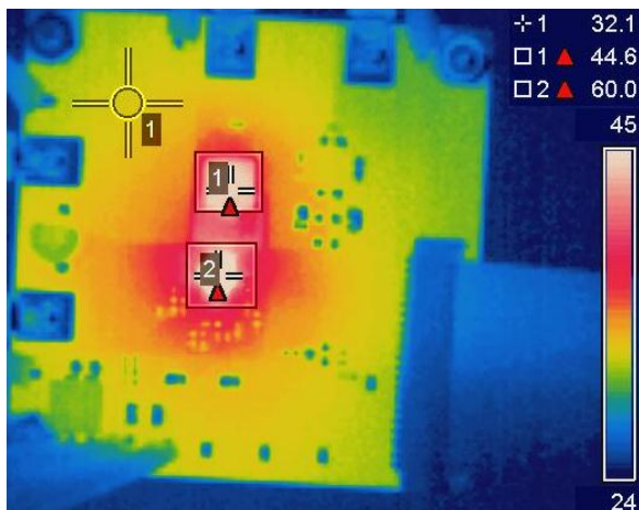
Figure 18: Thermal Image at V_{IN} = 12V , I_{OUT} = 6A (IR3863: 60^\circ C , Inductor: 45^\circ C , PCB: 32^\circ C )
