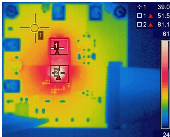
Figure 18: Thermal Image at V_{IN} = 12V , I_{OUT} = 10A (IR3865: 81°C, Inductor: 52°C, PCB: 39°C)
