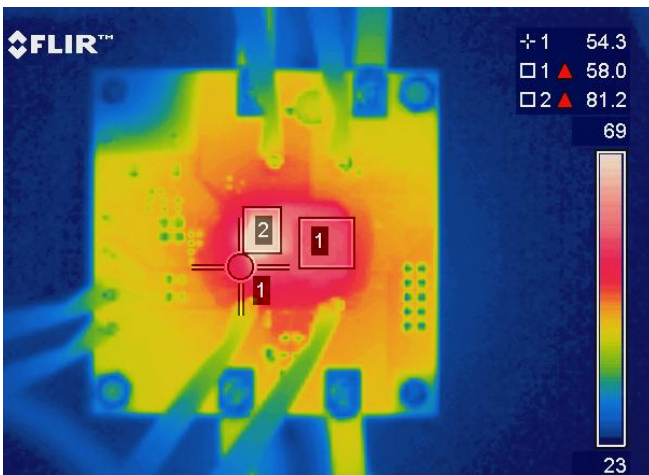
Figure 16: Thermal Image at I OUT = 12A (IR3876: 81°C, Inductor: 58°C, PCB: 54°C)
