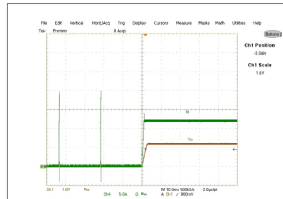
Figure 35: Short Circuit Recovery, Ch 1 :Vout, Ch 4 :Iout (5A/Div)
