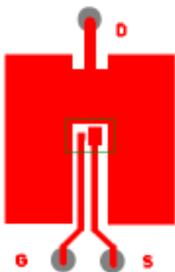
⑥ Surface mounted on 1 in. square Cu board (still air).
