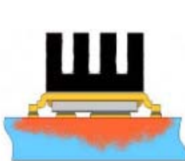
⑥ Mounted on minimum footprint full size board with metalized back and with small clip heatsink. (still air)
